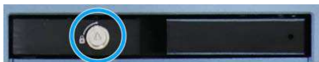
2.5" HDD/ SSD slot lock
