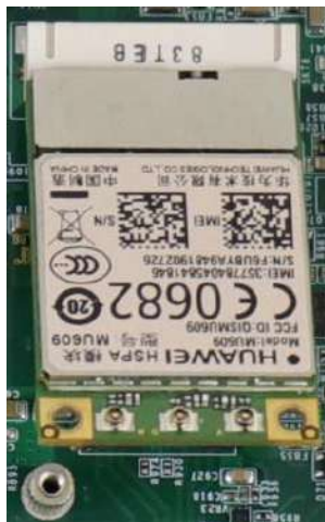
Insert on 45 degree angle
